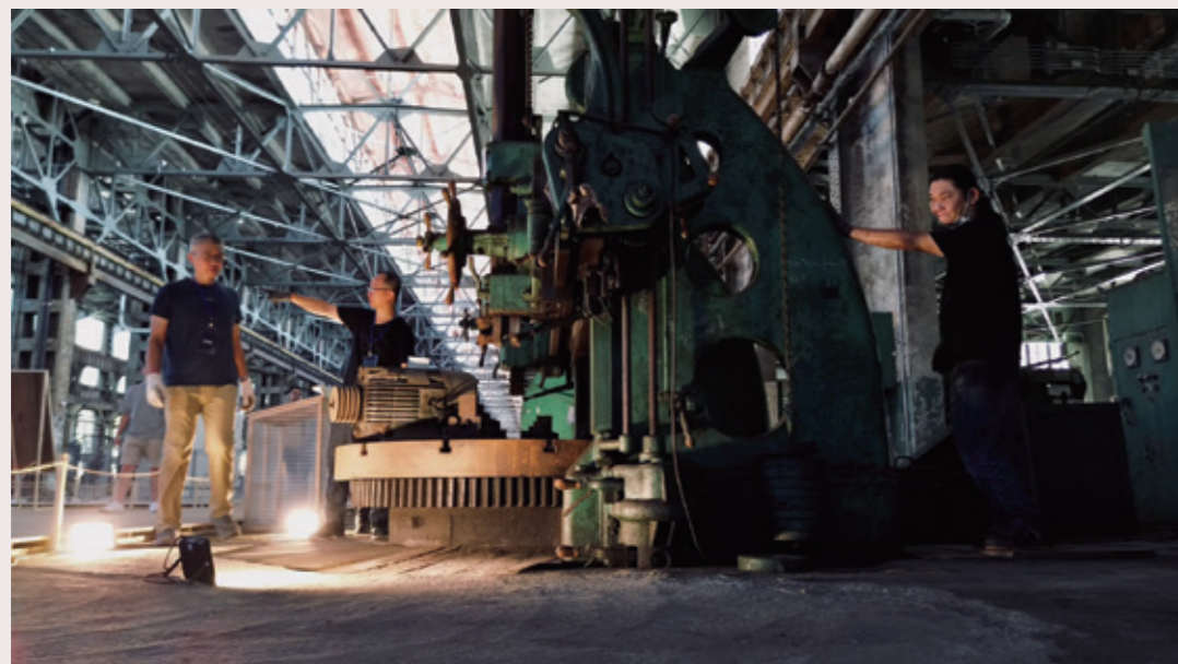
於鐵道博物館籌備處進行日治時期立式鏟床作動測試。 Conducting operational testing of the Japanese colonial period vertical boring machine at the Preparatory Office of the Railway Museum.
