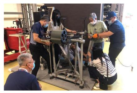
Transport of mechanical seismograph Invite experts to provide guidance for assembly and repair seismographs
