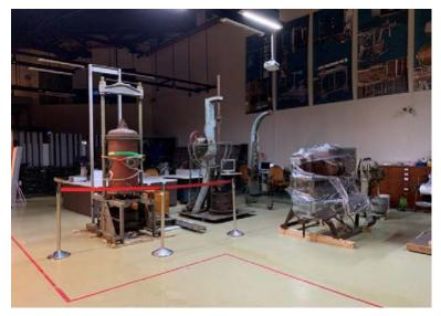
Large scale triaxial compression for the construction of Zengwen Reservoir
