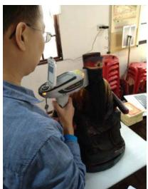
X-ray fluorescence (XRF) analyzer for detecting the paint ingredients of the faces of god statues
